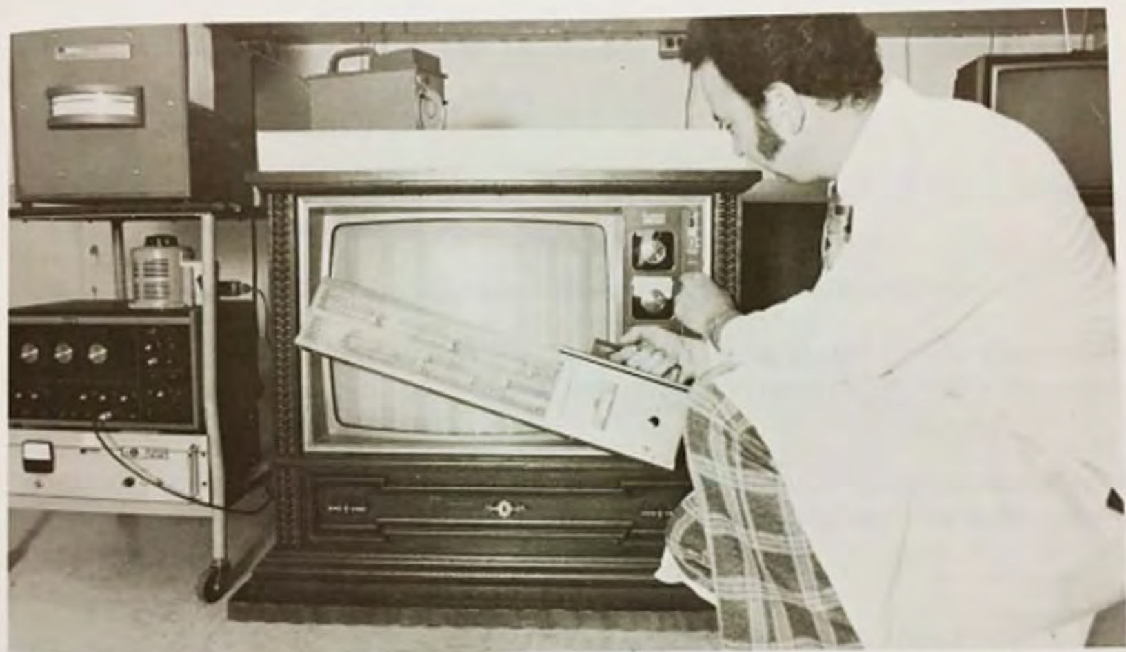
Technician checks x-ray emissions from color television receiver using Bureau-developed survey meter as part of overall laboratory product testing program.
